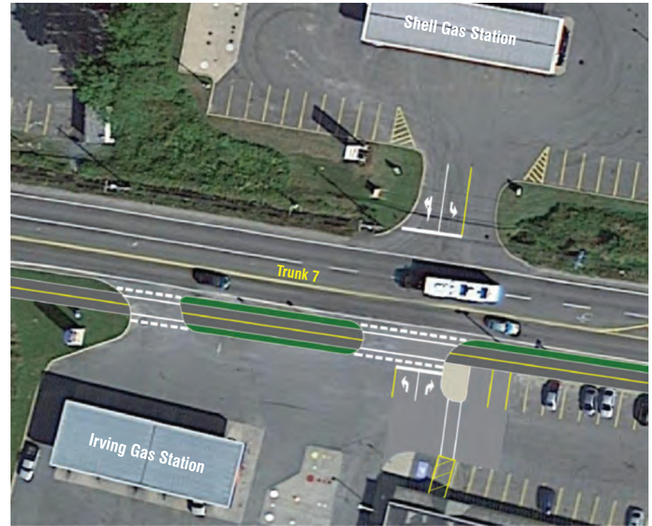
Conceptual sketch of recommended access management improvements. Note that a vehicle turning analysis should be complete as part of functional design recommendations.
